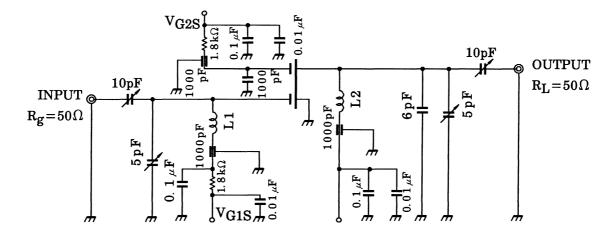
L1: 1 mm $\phi$  silver plated copper wire, 2 turns, 8 mm ID
